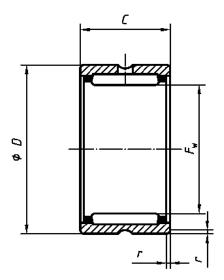
NOTE Needle roller bearings can be equipped with or without cage, with one row or two rows of needle roller and with or without lubrication groove and lubrication holes in the outer ring.
